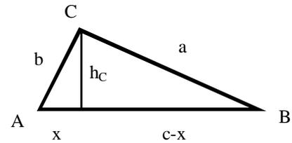
$$\left. \begin{array}{l} a^2 = h_C^2 + (c-x)^2 \\ h_C^2 = b^2 - x^2 \\ x = b \cdot \cos A \end{array} \right\} a^2 = b^2 - x^2 + c^2 + x^2 - 2cx = b^2 + c^2 - 2cx = b^2 + c^2 - 2cb \cdot \cos A$$
